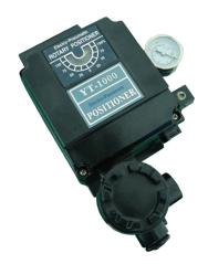
YT-1000R Electro-Pneumatic positioner is used for operation of pneumatic rotary valve actuator by means of electrical controller of control systems with an analog output signal of DC 4 to 20mA or split ranges.
